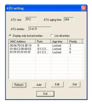
The Address Translation Unit (ATU) performs MAC address searching, learning, and aging functions for all ports of the IntelliJack. By default, the ATU table allows a total of 512 entries and an aging time is 304 seconds for each entry. These settings (ATU, ATU aging time, and ATU entries) are fixed and not editable.
